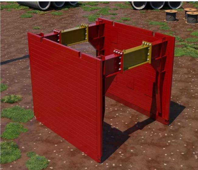
7. Once the box is fully assembled then it can be lifted into a vertical position ready for install into the trench. The box should not be left in a vertical position unless it is being lifted directly into the trench as it may become unstable due to changing ground conditions and high winds.
