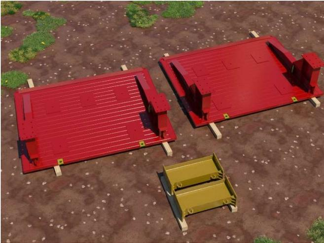
1. Commence by laying panels and struts on timber skids, with the panel strut connections facing skyward. Ensure all required strut components are present.
